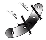
Install wood chip sock perpendicular to flow with ends curled slightly upstream to prevent high water from going around the ends. Slow and spread water to reduce channeling and erosion.
